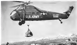
45 TONS PER HOUR —In northern Norway, pilots of the U. S. Army's 6th Helicopter Battalion carried loads of building materials, steel, electronic equipment, and even dynamite to mountain-top sites of micro-wave relay stations. The HO4S-1 (Sikorsky S-56) delivered their cargo at the rate of 1½ tons every 2 minutes.
